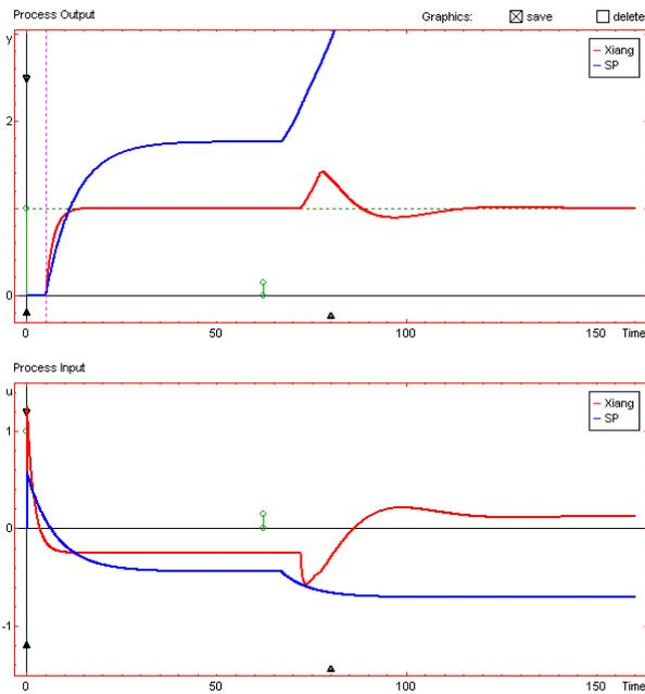
Fig. 6. Output response of the Smith Predictor and Xiang schemes for a unstable system and load disturbance of 0.1 at  $t = 55$ .
