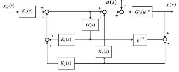
Fig. 3. Xiang DTC structure.
