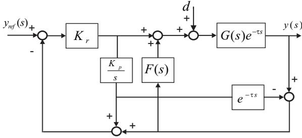
Fig. 2. Matausek DTC structure.
