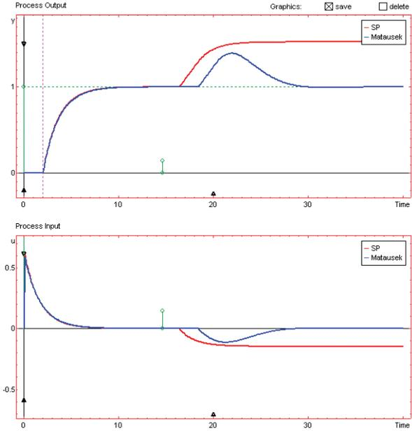
Fig. 5. Output response of the Smith and Matausek schemes for a step load disturbance of 0.1 at  $t = 15$ .
